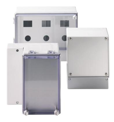
The instrumentation compartment in the standard model is covered with a transparent, hinged cover; quick release screws, which are available as an accessory, make opening of the cover even easier. The degree of protection is IP54.
